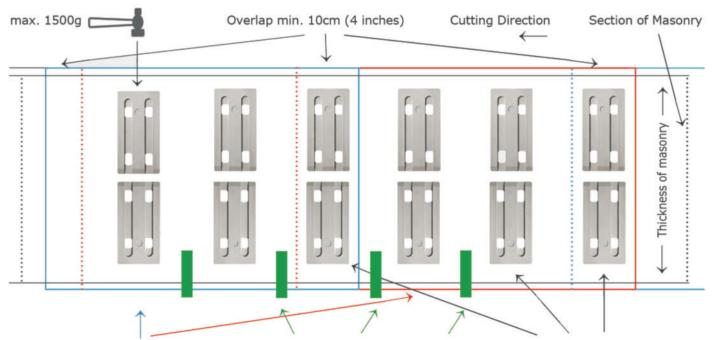
Insulating foils must always overlap 10 cm (4 inches) min. Prior to placing the foil, the saw cutting area must be cleaned using a special joint cleaner, removing any debris or loose joint material. A severely jagged wall surface can be levelled off with a thin layer of cement mortar before the foil is placed. When cutting the foil the required thickness of the plaster (1-2 cm) must be taken into consideration.
